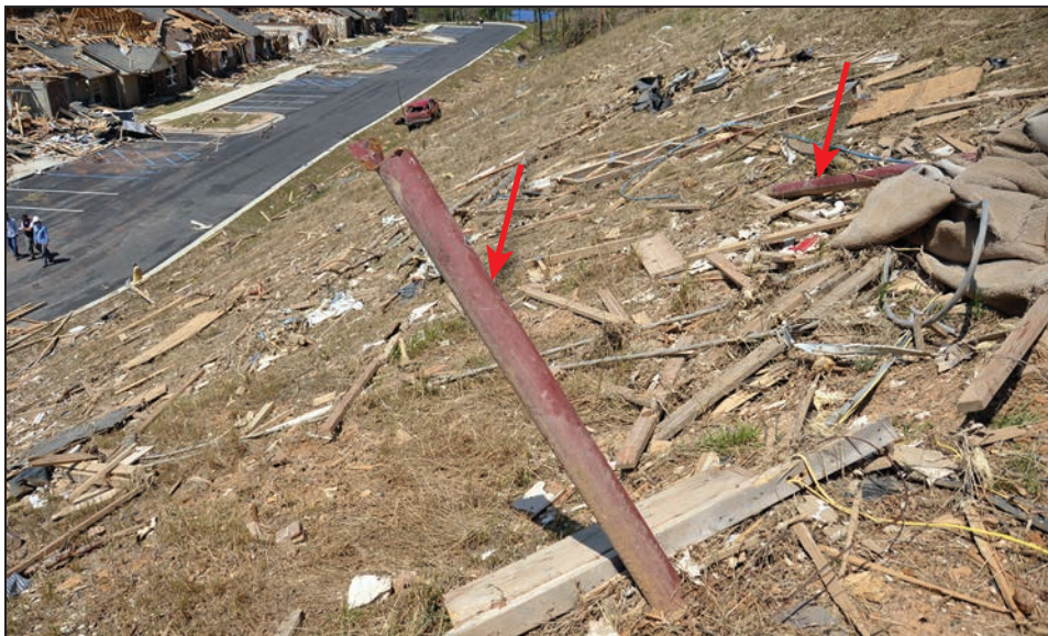
Figure B8-14. Steel porch column debris from an apartment complex where columns that were 7 feet 9 inches long and 4¼ inches in diameter (see red arrows) had a significant upward trajectory and flew approximately 230 feet (Tuscaloosa, AL, 2011 tornado)
